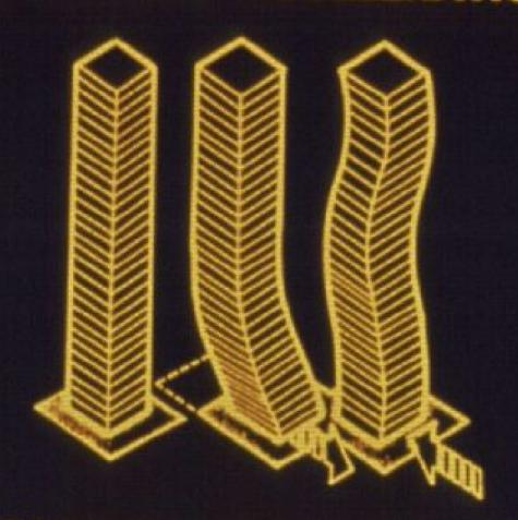
AT THE SAME TIME THAT THE UPPER PART OF THE STRUCTURE BEGINS TO MOVE TO CATCH UP WITH THE INITIAL DISPLACEMENT, THE GROUND MOTION REVERSES ITSELF.
