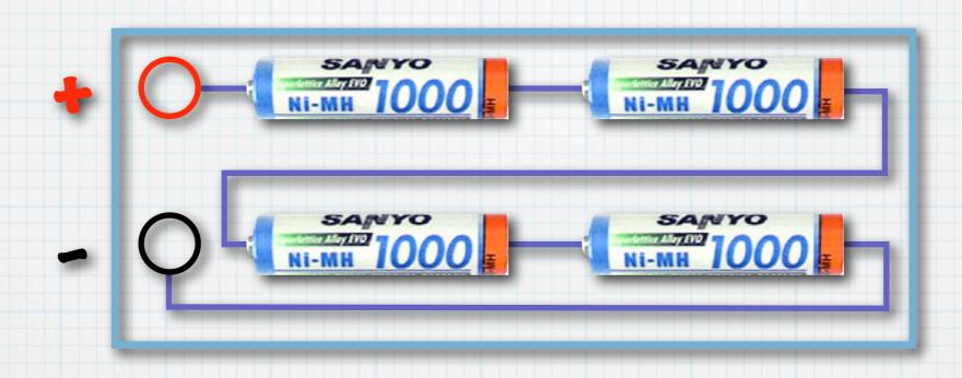
Made up of multiple cells in series
