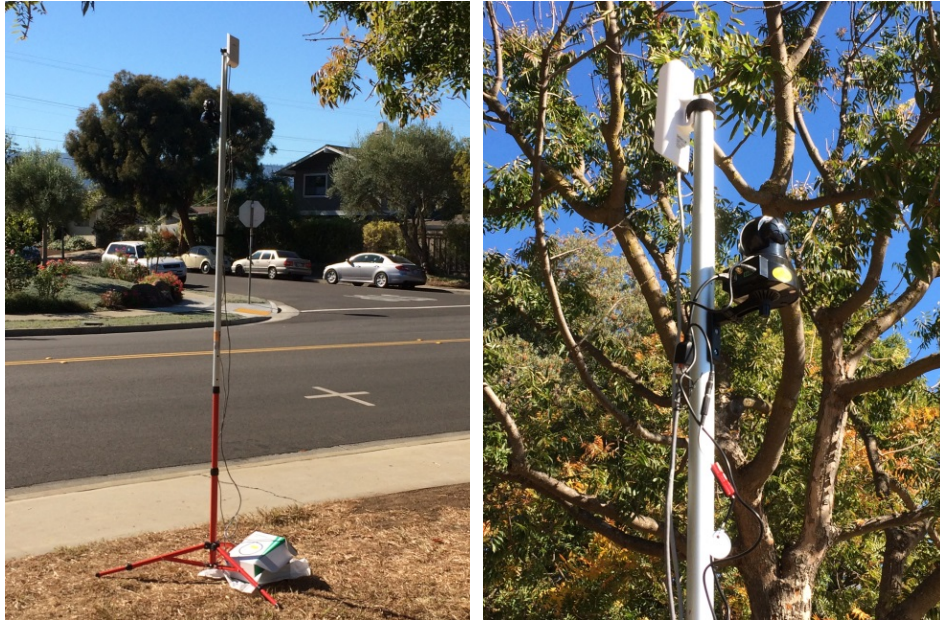
A 12vdc 12Ah battery is located in the box at the base of the mast. The box also holds the POE injector for the Ubiquiti as well as the 12vdc to 5vdc adaptor for the camera.
