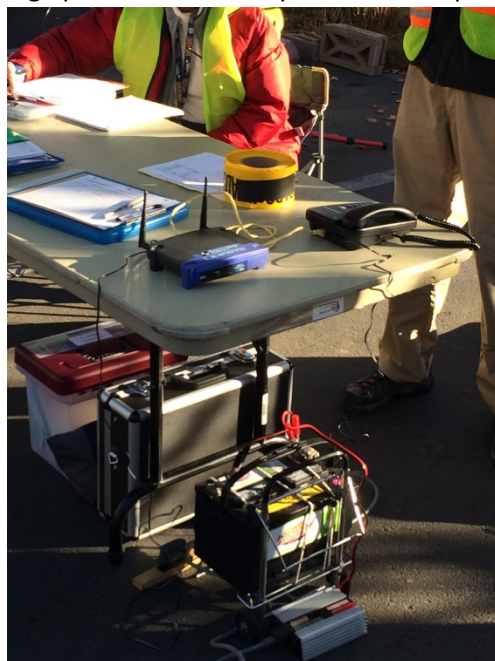
Skip's 75 Ah battery sitting on a the luggage cart next to the inverter.
