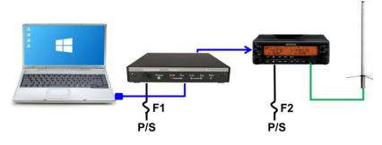
1. Connections: Confirm that all packet components are correctly cabled.
